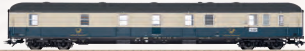
42851 Type Post mr-a Railroad Mail Car – Use the DC wheelset E700580 for the exchange
