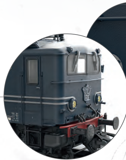
With original locomotive superstructure from the 1st series without front reinforcement ("Botsneus")
