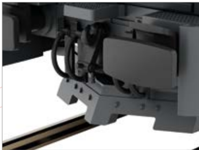
■ Buffer beam completely covered
