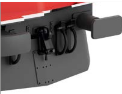
■ Buffer beam can be fully retrofitted
